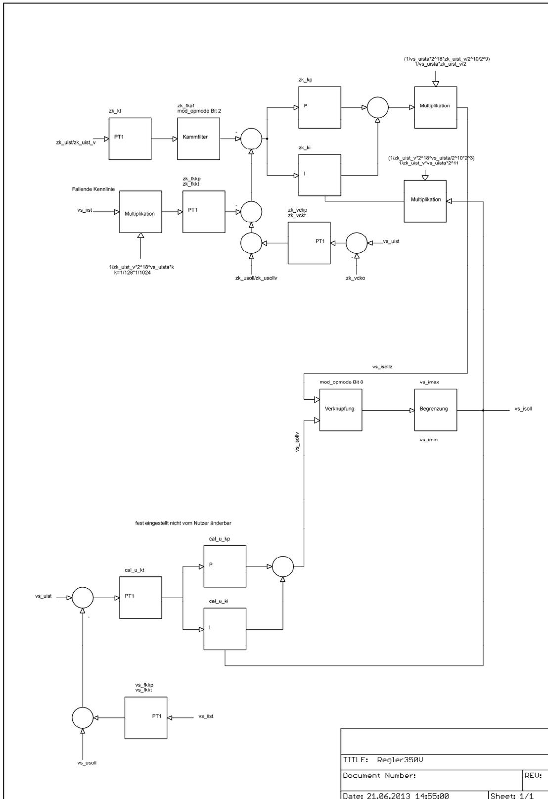
**Fig. 5: Block diagram of the voltage regulators**
