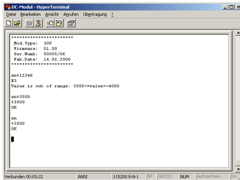
**Fig. 6:** *Module parameterization by means of terminal software*
