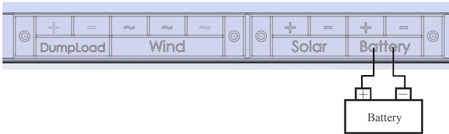
Battery wiring(the positive and negative cannot be reversed)
