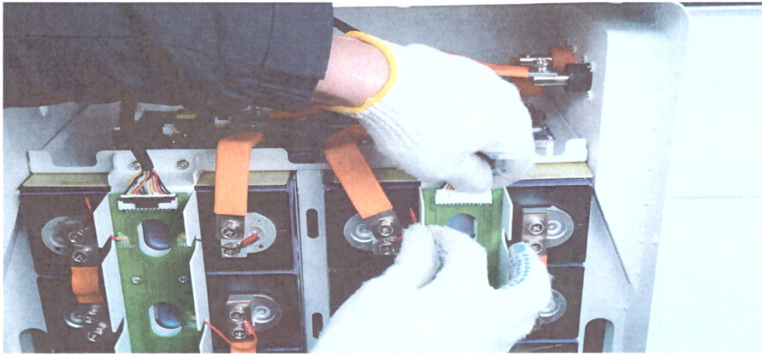
15. Connect the BMS wires(white)
