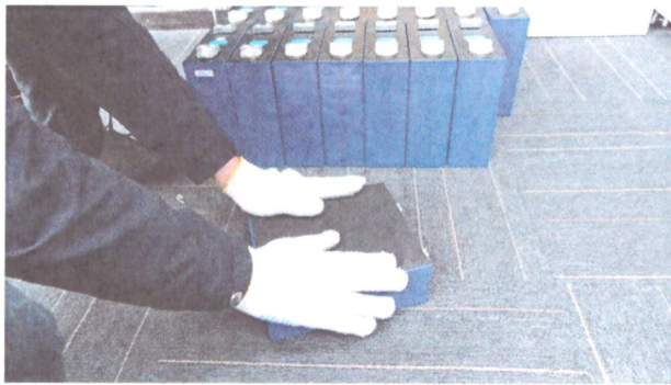
3. Stick on the EVA tapes, Please notice, if your cells are swollen , we don't recommend sticking the EVA tapes on.
