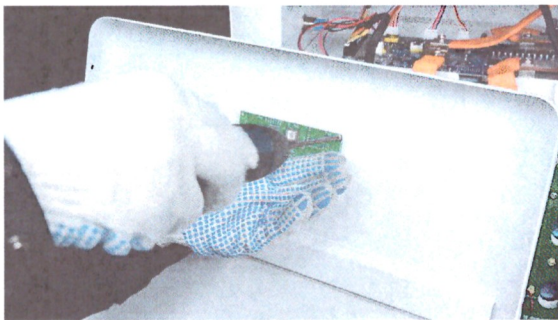
17. Fasten the LCD screen with screws
