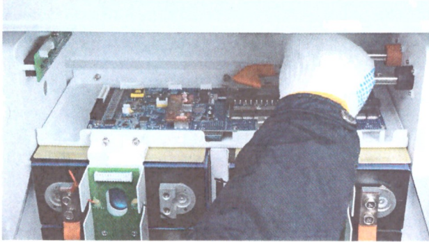
11. Fasten LCD screen with M3*8 screws
