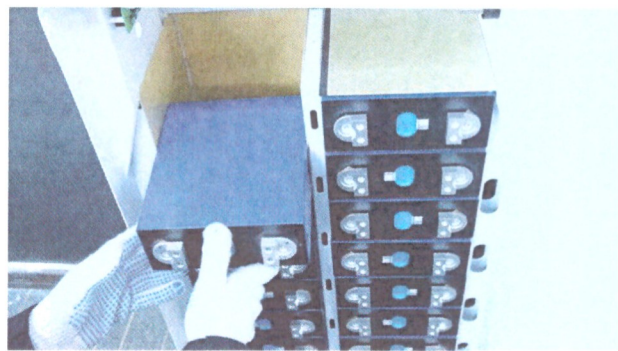
4. Put on the epoxy boards, and put the cells one by one , each cell has one epoxy board between
