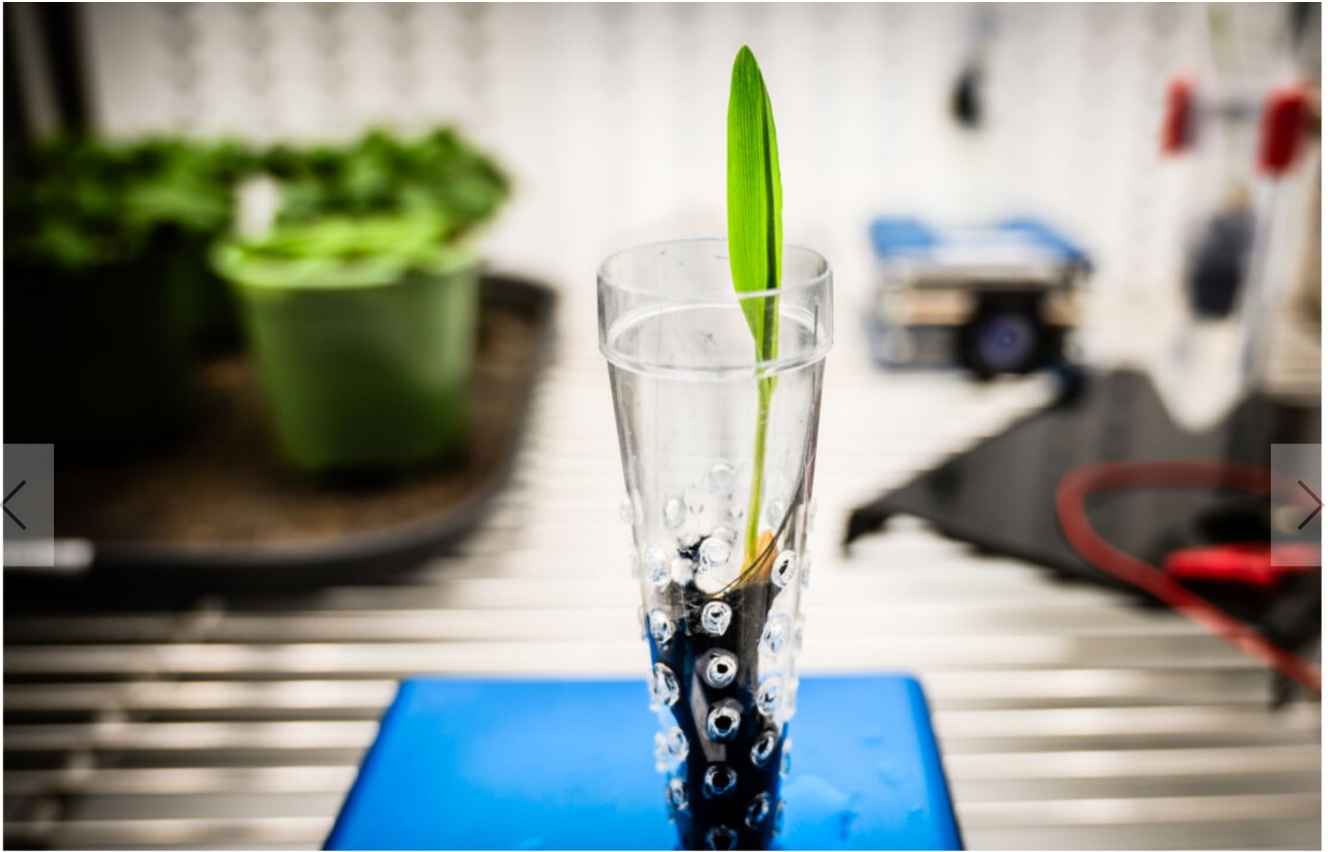
The eSoil, an electronic soil developed at the Electronic Plants group, is used to apply electricity to plants and accelerate t © Thor Balkhed
