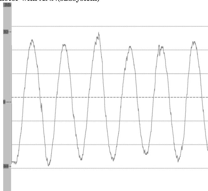
**Fig.10. Sinusoidal Hardware Output after filter (Voltage vs time)**
