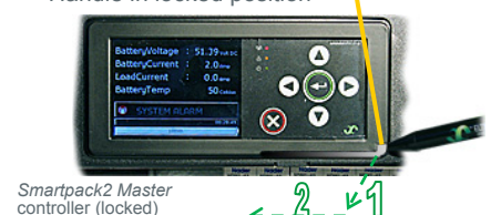
Handle in locked position
