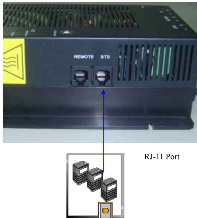
Figure 1 – 12: Install BTS
