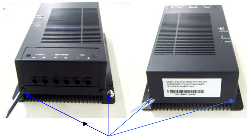
Figure 1 – 4: Removing the topcover
