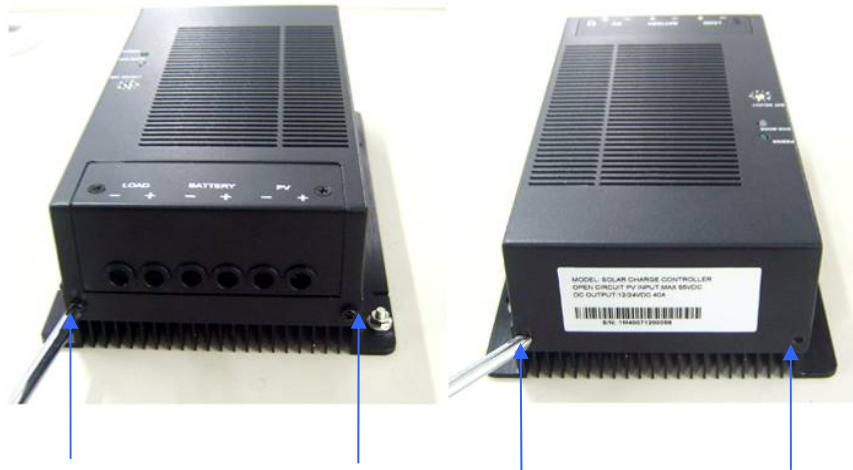
Figure 1 – 13: Reinstalling the faceplate
