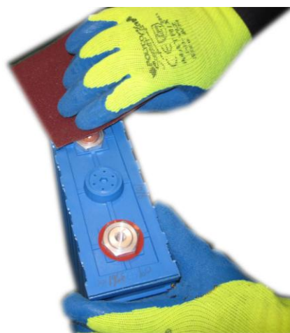
Picture 3.2.4.2: Sanding the battery
