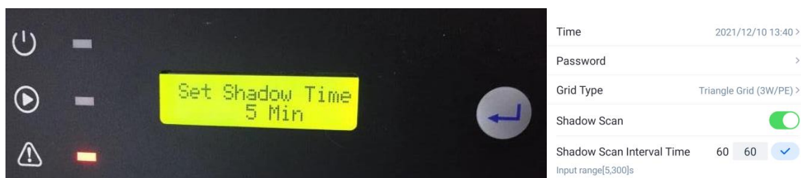
Fig 8. Setting Shadow Scan Interval Time on inverter display or SolarGo
